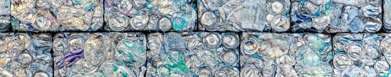
Crushed aluminum cans recycled into building blocks. Credit: iStockphoto/Gary Kavanagh
